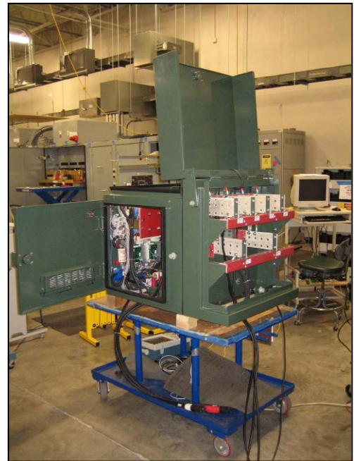
Figure 6: S&C 25 kW CES Unit Under Development
