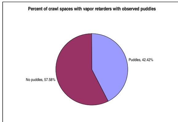
**FIGURE 23** Due to bulk water infiltration or significant dripping from condensation, water can pool on the surface of the ground vapor retarder
