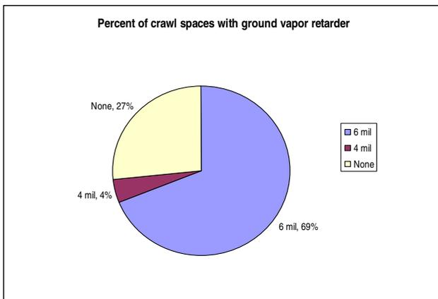
**FIGURE 19** Classification of crawl space vapor retarder condition
