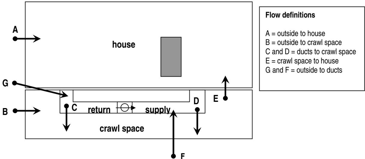
**FIGURE 3 Crawl space blower door set up**
