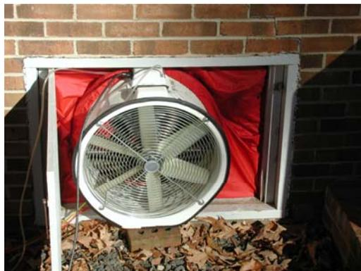
**FIGURE 4 House blower door set up**
