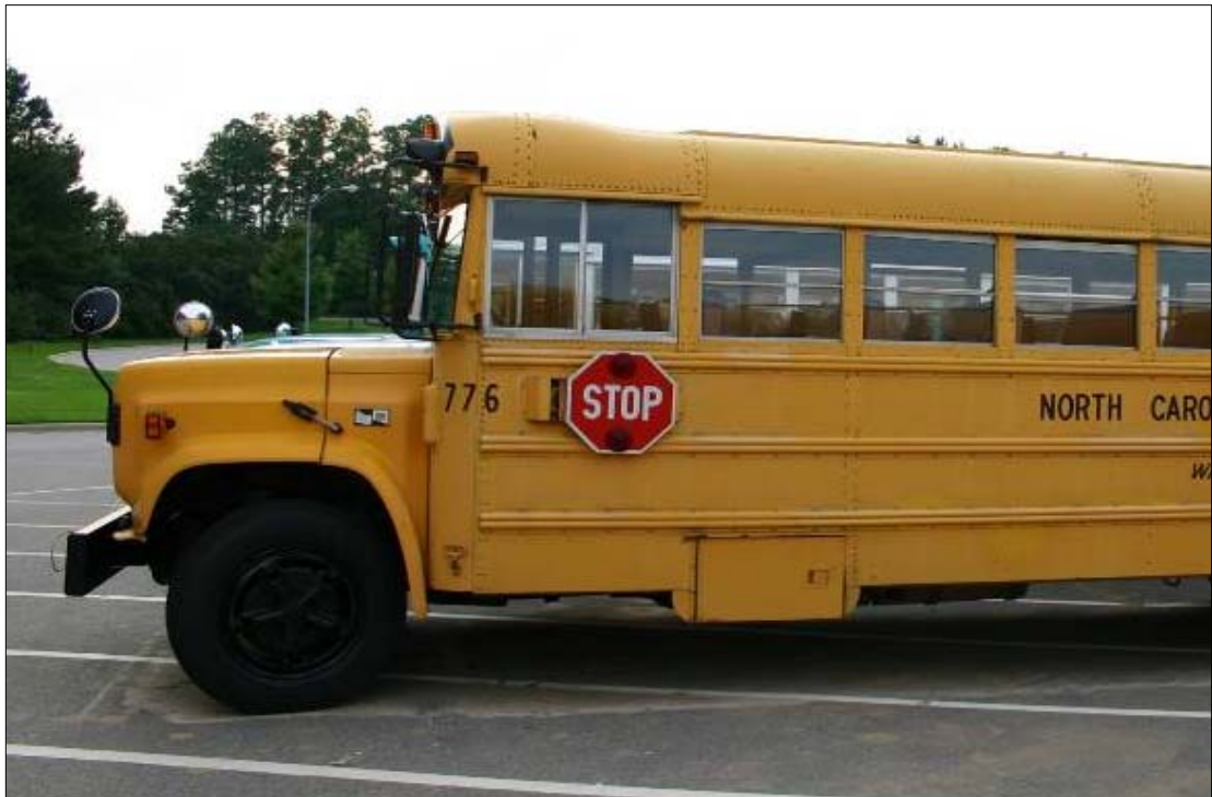
Type C school buses are the most common and are often referred to as “conventional” buses. The Hybrid Electric School Bus Project (HESB) focuses on this type of bus.
