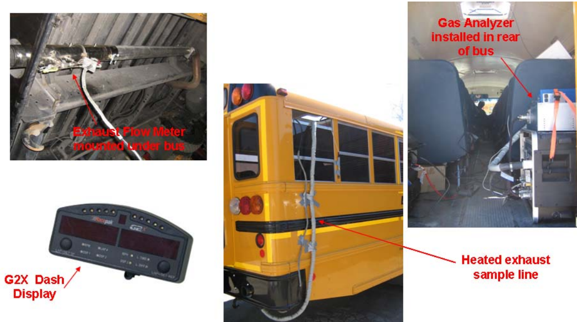
Figure 2-1 Emissions Test Equipment Installed in a Bus
